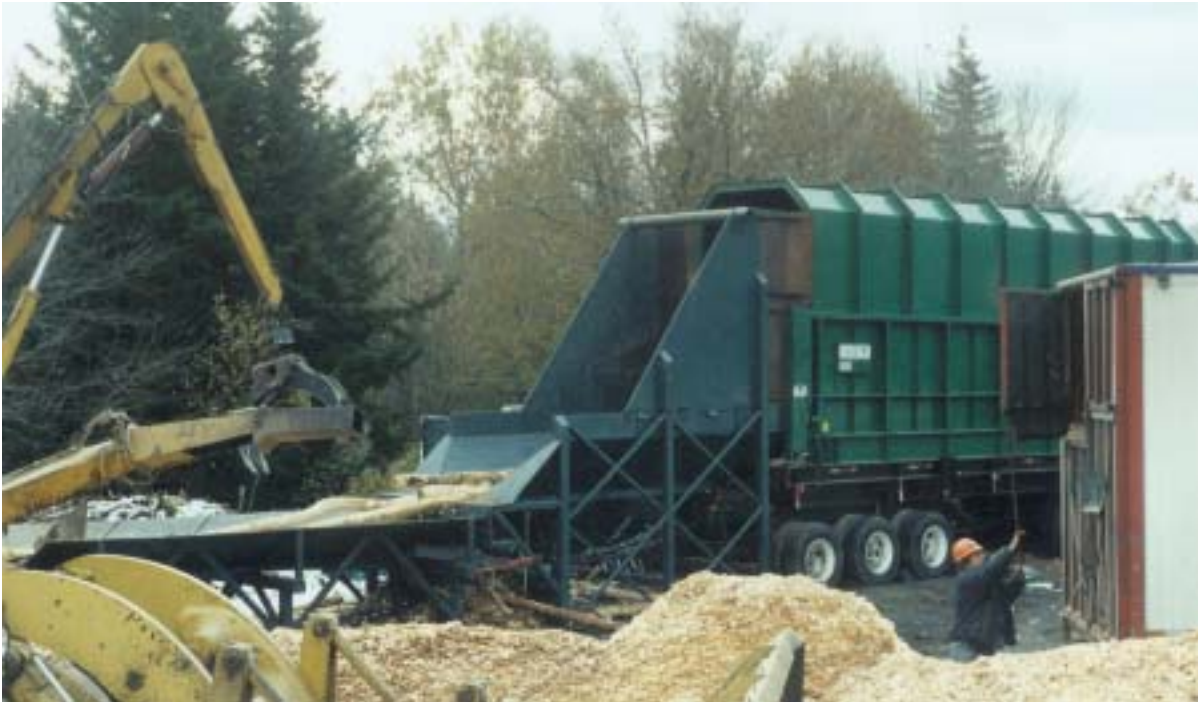
This Fuji-King Debarker supports a portable chipping operation near Liverpool, Nova Scotia
